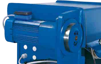
Cross travel drive Two compact epicyclic reduction gears with pole-changing brake motors directly drive two wheels.
