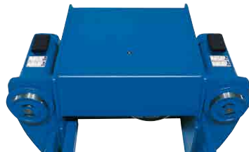
Cross travel trolley Hoist trolleys are fitted with four flanged wheels with permanently lubricated roller bearings, designed for use on tracks with parallel flanges. Wheels for tracks with inclined flanges are available as an option.
