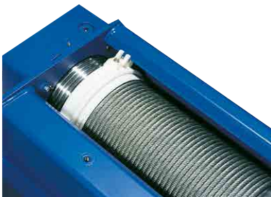
Rope guide A resilient low-friction plastic rope guide designed as an expanding ring provides positive guidance for the rope. The rope guide also reduces wear on the rope and rope drum. It is also easy to install, reducing maintenance requirements for the unit as a whole.
