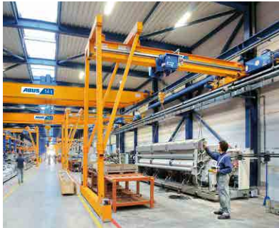
The ABUS single girder semi-goliath crane is designed for spans up to 15 m and Safe Working Loads up to 10 tonnes.
