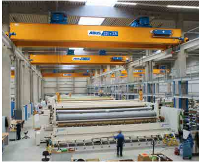
ABUS double girder travelling cranes achieve the maximum load capacity of up to 120 tonnes. They are available in various configurations and feature the versatility required for additional requirements. For example, higher crane travel speeds, maintenance walkways, trolleys with service platforms and auxiliary hoists are all features which can easily be implemented.
