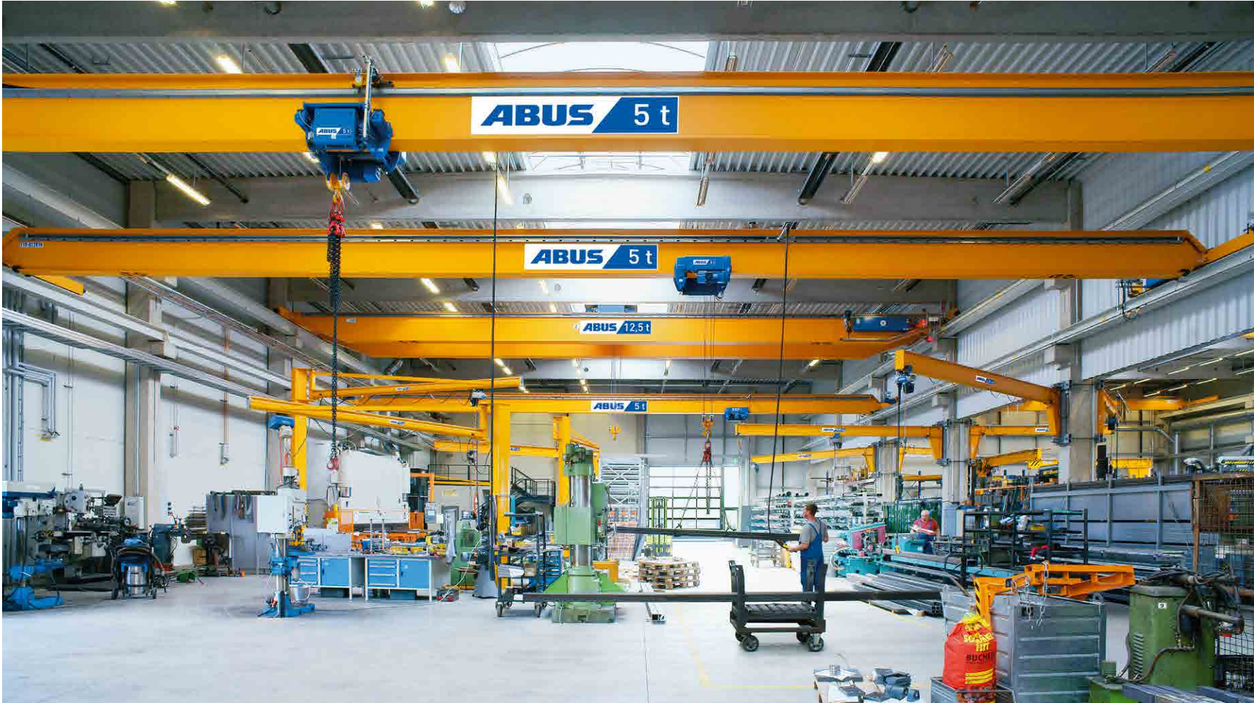
ABUS single girder wall travelling cranes and ABUS single girder semi-goliath cranes are installed on a separate track below other types of travelling crane. They are the ideal solution for serving several working areas at the same time. The ABUS single girder wall travelling crane is designed for spans up to 12 m and load capacities up to 5 tonnes.
