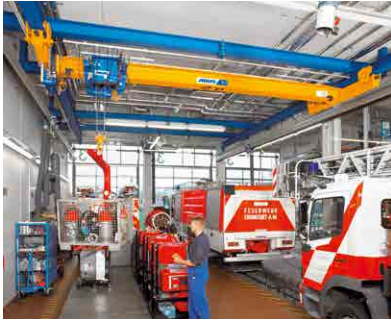
ABUS underslung travelling cranes are installed on ceiling mounted tracks rather than free standing or building columns. Advantageous side approach dimensions allow the optimum use of the entire width of the production.
