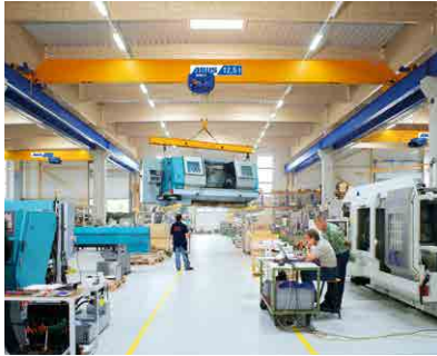
ABUS single girder travelling cranes ensure efficient material handling even where very little space is available in production halls or warehouses. ABUS single girder travelling cranes are available with rolled section or box girders. Each model is available in different girder connection versions to allow a space-saving configuration and an optimised highest hook position.
