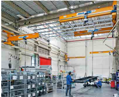
ABUS single girder wall travelling cranes and ABUS single girder semi-goliath cranes are installed on a separate track below other types of travelling crane. They are the ideal solution for serving several working areas at the same time. The ABUS single girder wall travelling crane is designed for spans up to 12 m and load capacities up to 5 tonnes.
